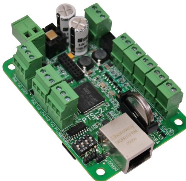
Variant of controller supply in a view of electrical board (PTS2-PCB-z or PTS2PRO-PCB-z)
