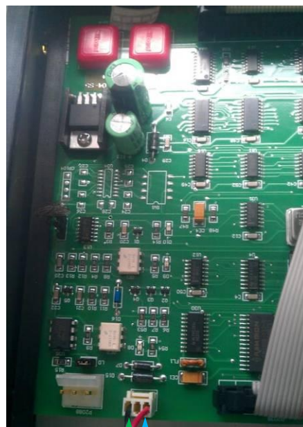
Gilbarco Endeavor dispenser board
